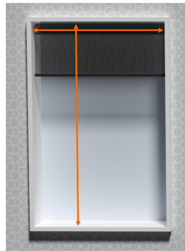
figure 1: measuring an inside fit roller blind
