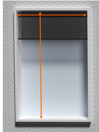
figure 1: measuring an inside fit roller blind
